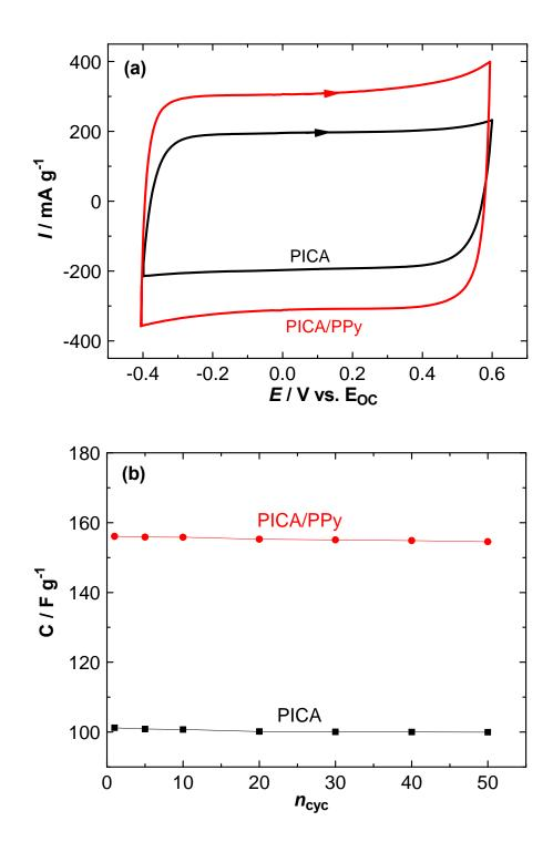
**Figure 2.** (a) Cyclic voltammograms of PICA and PICA/PPy electrodes at a  $2 \text{ mV s}^{-1}$  scan rate. The separator was impregnated with a  $1 \text{ M NaNO}_3$  aqueous electrolytic solution, (b) Evolution of the specific capacity of PICA and PICA/PPy electrodes as a function of the number of cyclic potential scans
