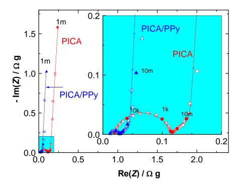
**Figure 3.** Comparison of the experimental EIS spectrum with the one calculated with the porous electrode model. The insert shows the HF part in enlarged scale (blue triangles and red circles : experimental data for PICA/PPy and PICA electrodes respectively, and + : calculated data with same color code)
