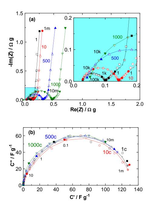
**Figure 6.** Ageing effect by potential cycling on the EIS spectra of PICA/PPy electrodes : (a) Nyquist-type plot (b) Cole-Cole plot
