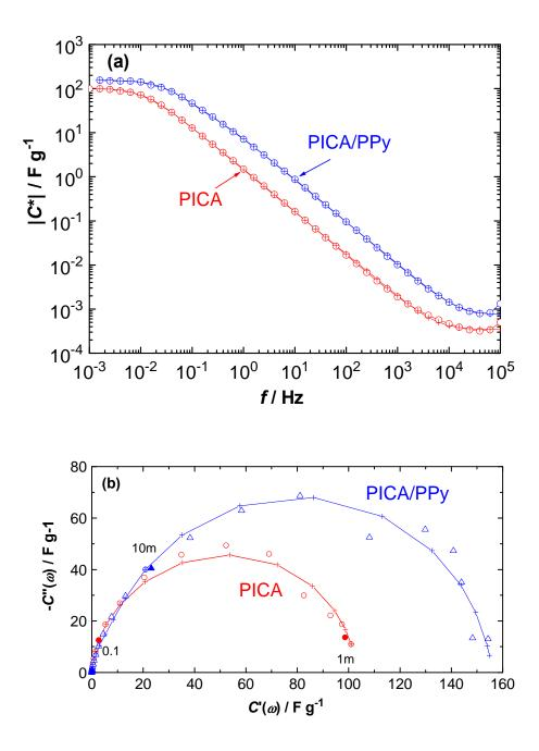
**Figure 5.** Evolution of the complex capacitance modulus as a function of frequency for the PICA (in red) and PICA/PPy (in blue) (a) Bode-type plot (b) Cole-Cole plot
