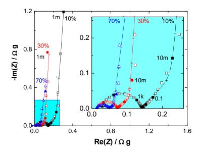
**Figure 7.** Comparison of the experimental impedance spectrum (experimental data) with the one calculated with the de Levie model for PICA / PPy electrodes for different mass percentages of PPy. The insert shows the HF part in enlarged scale (blue triangles and red circles : experimental data for PICA/PPy and PICA electrodes respectively, and + : calculated data with same color code)
