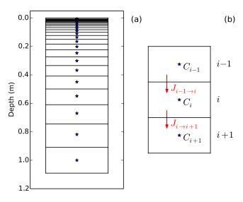
Figure 1. (a) The vertical finite-volume boxes and computational nodes (asterisk). (b) A schematic figure showing the diffusive fluxes (J) across boxes, which relate to concentration changes through mass balance.
