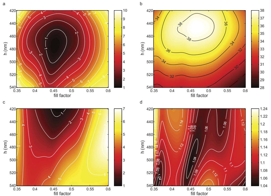
**Figure 4.** (a) Average of TE and TM efficiencies (%) in 0<sup>th</sup> transmitted order, (b) average of TE and TM efficiencies (%) in 1<sup>st</sup> transmitted order, (c) average of TE and TM efficiencies (%) in 2<sup>nd</sup> transmitted order. (d) Ellipticity of the beam diffracted into the 1<sup>st</sup> orders.
