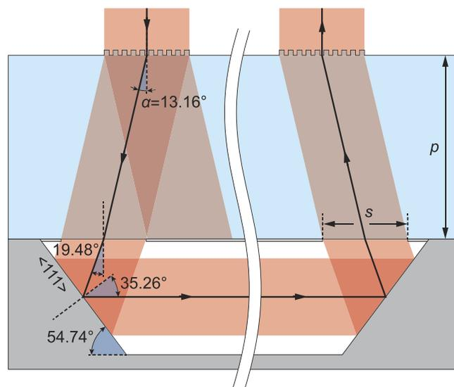
**Figure 3.** Routing of the beam in the cell.
