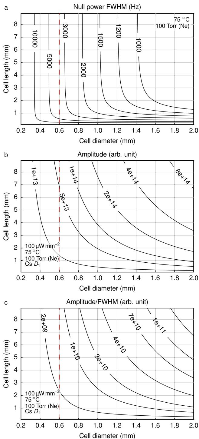
**Figure 7. Computed (a) CPT linewidth at null power, (b) amplitude and (c) resulting amplitude-to-linewidth ratio of CPT signals for different cell dimensions.** The cell temperature is 75 °C and the buffer gas (neon) pressure is 100 Torr.
