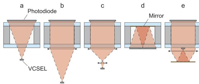
**Figure 1. Sketches of optical configurations (not to scale).** (a) Naturally diverging beam. (b) Simple collimation. (c) Collimation and reduction of the propagation length with a lens doublet. (d) Folded and diverging beam. (e) Collimation and reduction of the propagation length by beam folding using a mirror and a dual-focus lens.
