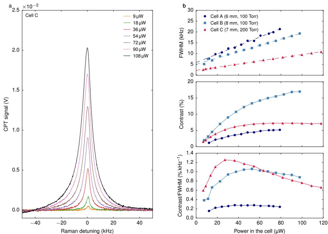
**Figure 8.** (a) CPT signals in cell C for different powers. The cell temperature is 75°C and the magnetic field magnitude is 20 μT. The background is removed for clarity (b) linewidth, contrast and contrast-to-linewidth ratio in different cells.
