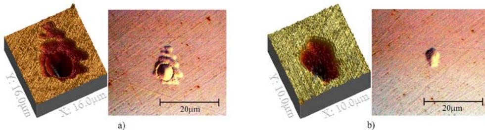
Fig. 2. Comparison of morphology of craters eroded in the  $\text{PbWO}_4$  sample at a fluence of (a) 35-fold and (b) 4-fold above the single-shot ablation threshold, as taken with AFM (left) and DIC (right) microscope.
