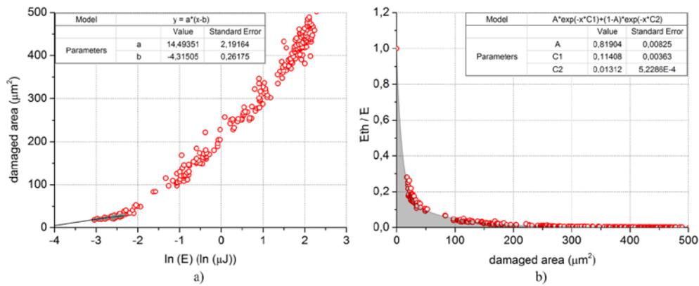
Fig. 4. (a) Liu's plot for PbWO<sub>4</sub> with determined threshold energy and (b) the corresponding normalized f-scan.
