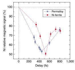
**Figure 5 | Time-dependent magnetic signal.** Ni demagnetization in the permalloy (blue squares) and the Ni-ferrite (red circles) samples at several delays  $\Delta t$  between probe and pump pulses ( $F=10~\text{mJ}~\text{cm}^{-2}$ ). Vertical error bars represent s.d. (see Methods). The maximum fluctuation in the pump-probe delay over the measurement duration ( $\pm 5~\text{fs}$ , see Methods) is smaller than the point width. Lines are a guide to the eye.
