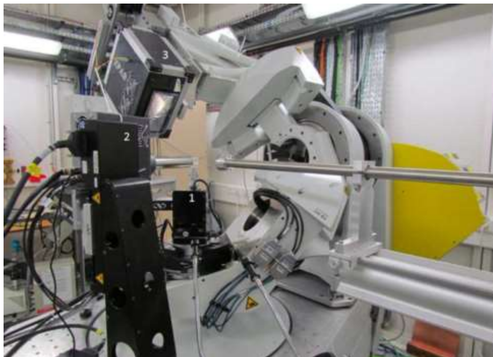
Figure 1: the 6+2 circles diffractometer in Kappa Geometry on DiffAbs beamline with (1) sample positioning using micrometric motorized tables, (2) SDD-4E detector for XRF measurements, (3) hybrid pixel area detector XPAD for XRD measurements.
