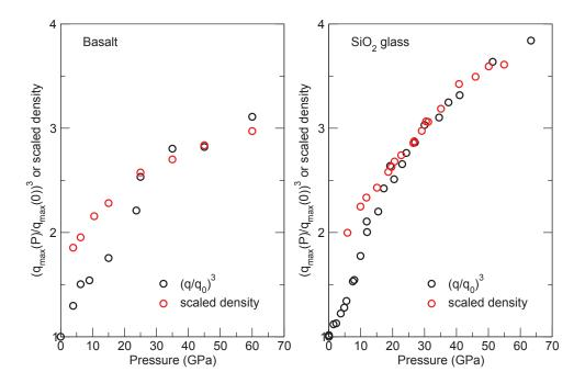
Figure 7: Evolution of the position of the first sharp diffraction peak  $(q_{max})$  with P compared to that of density scaled down to match the evolution of  $q_{max}(P)/q_{max}(0)$  at the highest P. For basalt,  $q_{max}$  values have been taken from Sanloup et al. (2013b), for SiO<sub>2</sub> glass, they are from Sato and Funamori (2010) and Inamura et al. (2004).
