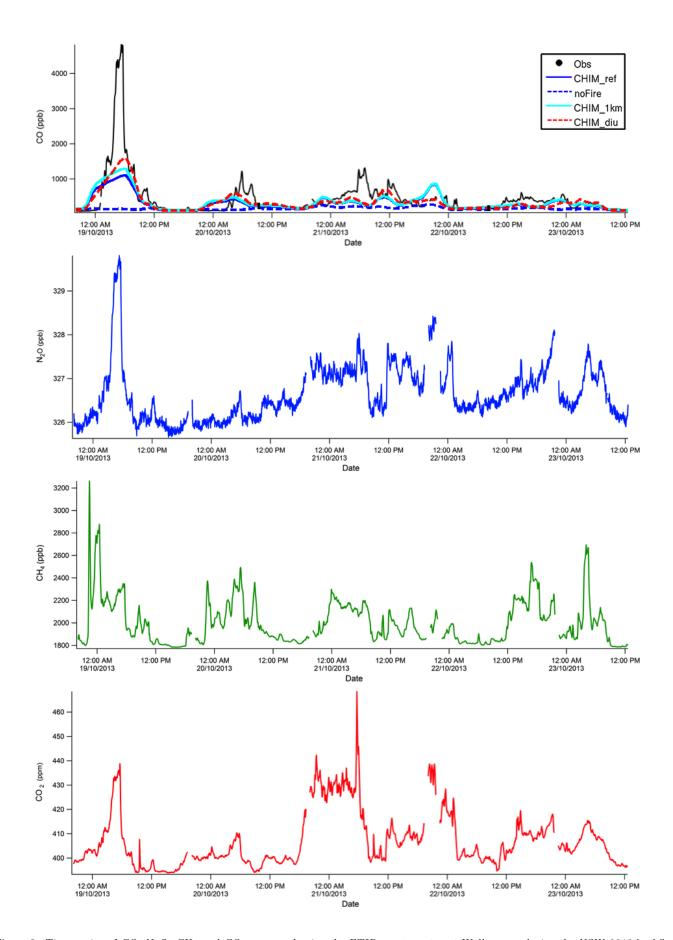
$Figure \ 2: \ \textit{Time-series of CO, N$_2O$, CH$_4$ and CO$_2$ measured using the FTIR spectrometer at Wollongong during the NSW 2013 bushfires. } \\$
