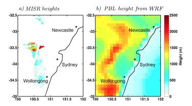
Figure 10: a) Top heights of the fire plume on the 20th of October, as derived from measurements by the MISR instrument onboard the Terra satellite (Level 2 "TOA/Cloud heights and Winds" product).
