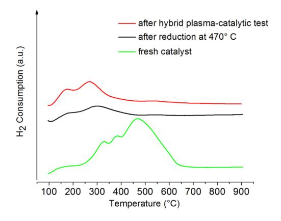
Fig. 9: Comparison of TPD profiles of the 15NiCZ5842 catalyst, fresh and after the 100 hours duration hybrid plasma-catalytic methanation test.
