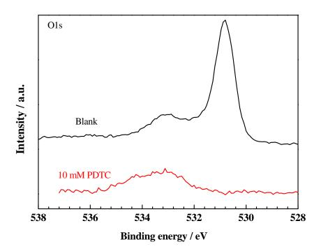
Figure 15: O1s spectra of Cu electrode after 24 h immersion in 0.2 g  $L^{-1}$  NaCl without or with 0.1 mM or 10 mM PDTC.
