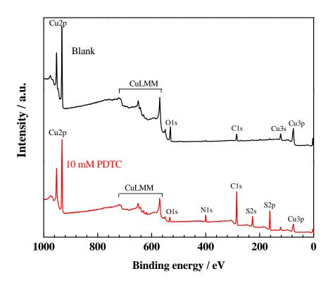
Figure 14: Survey XPS spectra of copper electrode after 24 h immersion in 0.2 g  $L^{-1}$  NaCl without or with 0.1 mM or 10 mM PDTC.
