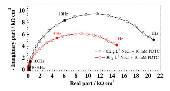
Figure 3: Nyquist diagrams of copper after 100 seconds exposure time in 0.2 g  $L^{-1}$  + 10 mM PDTC or 30 g  $L^{-1}$  + 10 mM PDTC; stationary electrode at 20°C.
