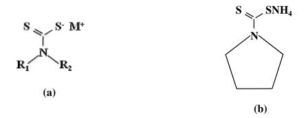
Figure 1: Structures of dialkyl dithiocarbamate (a) and ammonium pyrrolidine dithiocarbamate (b).
