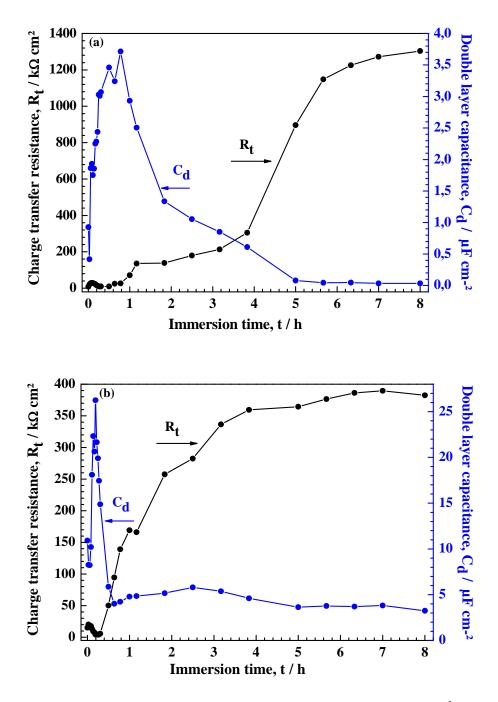
Figure 6:  $R_t$  and  $C_d$  change as a function of immersion period for  $Cu / 0.2 \text{ g L}^{-1} \text{ NaCl} + 10 \text{ mM PDTC}$  (a) and  $Cu / 30 \text{ g L}^{-1} \text{ NaCl} + 10 \text{ mM PDTC}$  (b); stationary electrode at 20°C.
