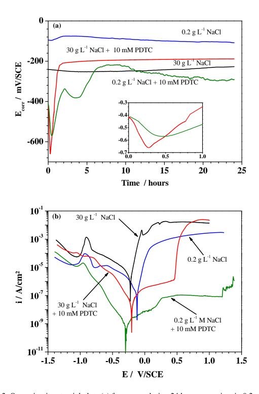
Figure 2: Open circuit potential plots (a) for copper during 24 h exposure time in 0.2 or 30 g  $L^{-1}$  NaCl without or with 10 mM PDTC and polarization plots (b) after exposure; stationary electrode at 20 °C.
