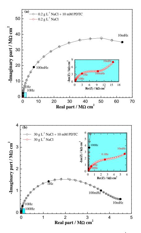
Figure 8: Nyquist diagrams of copper after 24 h exposure time in 0.2 g  $L^{-1}$  (a) or 30 g  $L^{-1}$  (b) without or with 10 mM PDTC; stationary electrode at 20°C. Symbols = experimental data; and crosses = calculated data.
