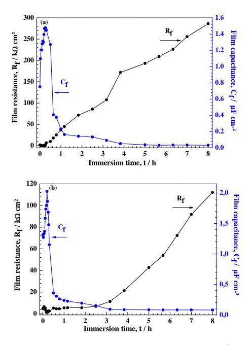
Figure 5:  $R_f$  and  $C_f$  change as a function of immersion period for  $Cu / 0.2 \text{ g L}^{-1} \text{ NaCl} + 10 \text{ mM PDTC}$  (a) and  $Cu / 30 \text{ g L}^{-1} \text{ NaCl} + 10 \text{ mM PDTC}$  (b); stationary electrode at 20°C.
