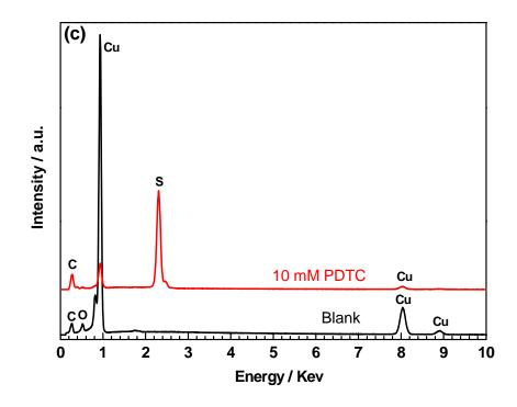
Figure 10: SEM images of copper surface after 24 h immersion time in 0.2 g  $L^{-1}$  NaCl without (a) and with 10 mM PDTC (b) and the corresponding EDX analysis (c).
