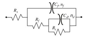
Figure 4: Electrical equivalent circuit to reproduce experimental impedance spectra for Cu electrode in 0.2 or 30 g  $L^{-1}$  NaCl without or with 10 mM PDTC for high and medium frequencies.
