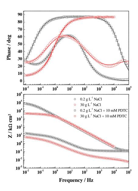
Figure 7: Bode diagrams of copper after 24 h exposure time in 0.2 or 30 g  $L^{-1}$  without or with 10 mM PDTC; stationary electrode at 20°C.
