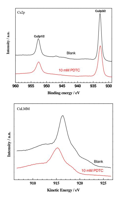
Figure 16: Cu2p and CuLMM spectra of Cu electrode after 24 h immersion in 0.2 g  $L^{-1}$  NaCl without or with 0.1 mM or 10 mM PDTC.
