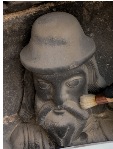
Fig. 1 Collecting powdery deposit sitting on the top of black crusts at Saint Denis Basilica.
