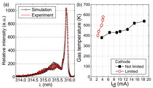
Figure 6. (a) Fit on the experimental spectra of the 1–3 band of the second positive system of nitrogen at 100 Torr and 15 mA providing  $T_g = 520$  K. (b) Gas temperature versus current at 100 Torr in helium for  $D_{LIM} = 1$  mm and for non limited cathode surface.
