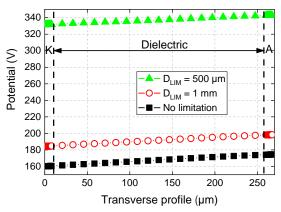
Figure 11. Simulation results for the potential profile along the central axis of the cavity for a cathode surface: (a) not limited, (b)  $D_{LIM} = 1 \text{ mm}$  and (c)  $D_{LIM} = 1 \text{ mm}$ .
