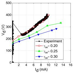
Figure 8. Experimental and simulated V-I curves for  $D_{LIM} = 1$  mm. The micro-discharge is operating in helium at 100 Torr and the best fit is obtained for  $\gamma_{se} = 0.2$ . The slope of the load line between points A and B corresponds to the value of the experimental ballast resistor: 40 k $\Omega$ .
