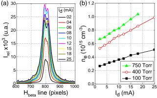
Figure 7. (a)  $H_{\theta}$  line profile in helium at 100 Torr for  $I_d = 2-25$  mA. (b) Electron number densities versus the operating current for a single microdischarge working at 100, 400 and 750 Torr in helium. The cavity diameter is approximately 260 µm.
