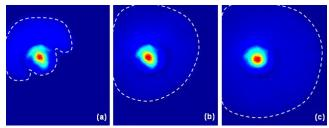
Figure 5. ICCD Pictures of the micro-discharge optical emission intensity on the cathode side (relative scale). The plasma increasingly spreads over the cathode surface as discharge current increases. (a)  $I_d = 5 \text{ mA}$ ; (b)  $I_d =$ 9 mA; (c)  $I_d = 20 \text{ mA}$ . The diameter of the MHC circular cavity is 260 µm.
