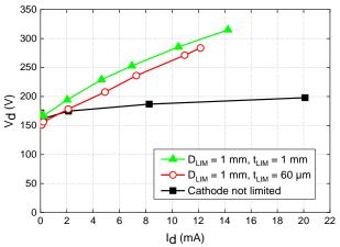
Figure 14. Simulated V-I curves of a microdischarge operating in helium at 100 Torr ( $D_{cav} = 260 \mu m$ ) for different dimensions of the limiting layer. The opening diameter of the limiting layer is 1 mm and its thickness is 60  $\mu m$  or 1 mm.
