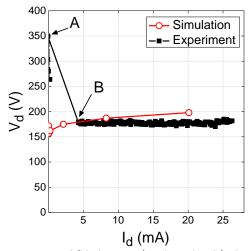
Figure 4. Experimental (black squares) and simulated (red circles) V-I curves for a micro-discharge generated in helium at 100 Torr. The microcavity has a diameter of  $260 \,\mu$ m and the cathode surface area is not limited. The solid line between points A and B helps to guide the eye showing the current increase and discharge voltage decrease which occurs at ignition. The simulation results were obtained for a value of the secondary electron emission coefficient of 0.3.
