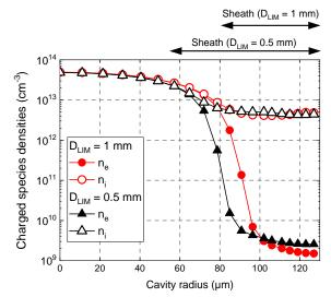
Figure 12. Simulated profiles of charged species densities along the radius of the cavity. The cathode surface is at 130  $\mu$ m and the discharge axis is at zero. Two cases are considered at 100 Torr in helium:  $D_{LIM} = 1$  mm and  $D_{LIM} = 500 \,\mu$ m, both for  $I_d = 5$  mA.
