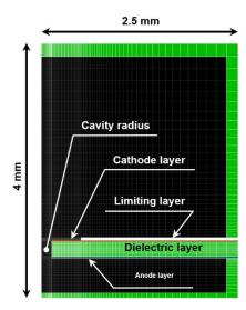
Figure 2. Computational domain of the MHC device. The axis of cylindrical symmetry is on the left and the computational grid is superimposed.
