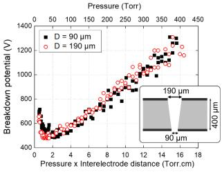
Figure 3. Paschen curves of a micro-hollow cathode and characteristic dimensions of the micro-cavity tested.
