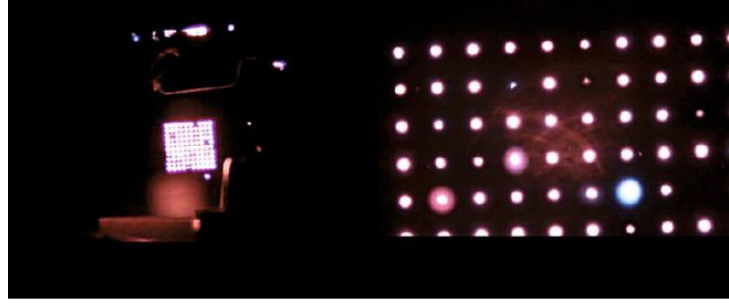
Fig. 10. (a) Picture of a 10 \times 10 micro-discharge array (50 \mu\text{m} diameter) operating in helium at 1000 torr for a total current of \sim 15 mA showing the main micro-discharges and some transient sparks which appear at the edges of the sample. (b) Picture taken in the same experimental conditions, but with a higher optical magnification.
