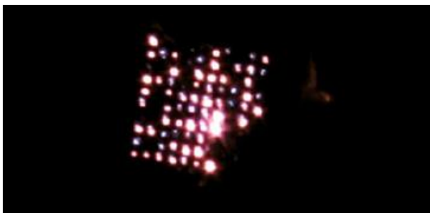
Fig. 9. Micro-discharge array at 1000 Torr in helium (100 μm diameter cavities) at 20 mA.
