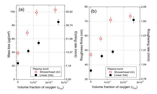
Figure 7. (a) Mass losses and etching rate vs the volume fraction of  $O_2$  (b)  $R_{rms}$  values and roughening rate vs the volume fraction of  $O_2$  for LDPE surfaces treated by the linear and showerhead plasma torches ( $P_{RF}$ =90W, t = 30 s, g = 2 mm).
