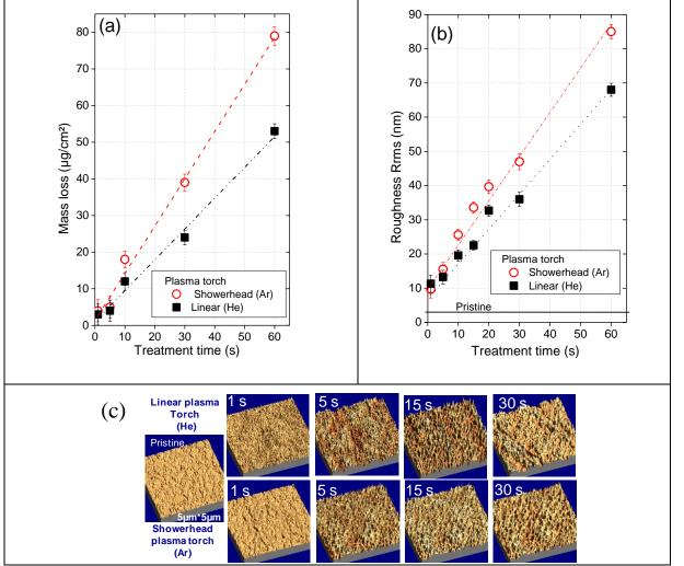
Figure 3. (a) Mass losses, (b) Root mean squared roughness ( $R_{rms}$ ) and (c) Tridimensional AFM images (5\*5 $\mu$ m<sup>2</sup>) vs. treatment time between 1 s and 60 s, using linear (He) and showerhead (Ar) plasma torches (g = 2 mm,  $P_{RF}$ =90W).
