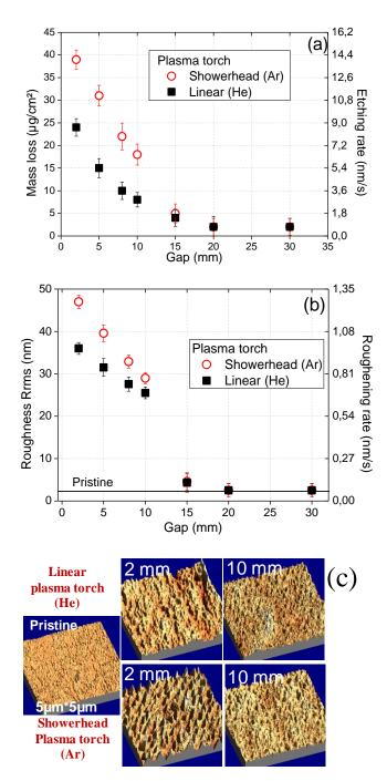
Figure 5. (a) Mass losses and etching rate, (b) Root mean squared roughness ( $R_{rms}$ ) and roughening rate (c) Tridimensional AFM images (5\*5 $\mu$ m<sup>2</sup>) vs. gap between 2nm and 30nm, for treatments achieved with the linear (He) and showerhead (Ar) plasma torches (t = 30s,  $P_{RF}$ =90W).
