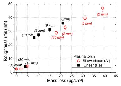
Figure 9. Surface roughness versus the mass loss of LDPE films treated by the linear (pure He) and showerhead (pure Ar) plasma torches, as in the Figure 5 (t=30s,  $P_{RF}$ =90W). Numbers in parentheses correspond to the values of the gaps.
