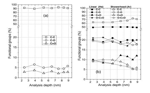
Figure 8. Depth profiles of the C-C, C-O, C=O and O-C=O chemical bonds for (a) native LDPE sample and (b) LDPE samples treated by the linear and showerhead plasma torches ( $P_{RF}$ =90W, t=30 s, g=2 mm).
