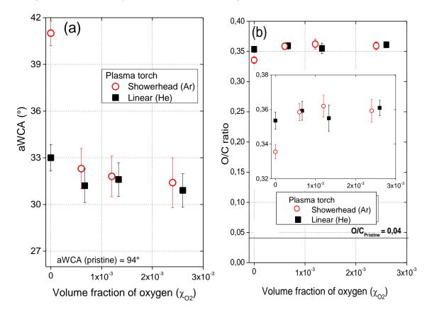
Figure 6. Variations of the (a) aWCA and (b) O/C ratio vs. volume fraction of oxygen (P<sub>RF</sub>=90W, t =30 s, g=2 mm)for LDPE surfaces treated by the linear and showerhead plasma torches,.
