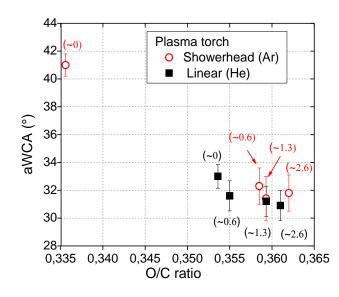
Figure 10. Advancing WCA versus the O/C ratio of LDPE films treated by the linear and showerhead plasma torches, from Figure 6 (t=30s,  $P_{RF}$ =90W, gap = 2 mm). The numbers in parenthesis correspond to 10<sup>-3</sup> of the O<sub>2</sub> volume fraction.
