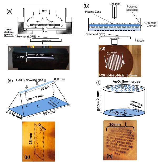
Figure 1. Schematic diagrams of the (a) linear plasma torch (supplied in helium) and (b) showerhead plasma torch (supplied in argon). Pictures of the (c) He post-discharge and (d) Ar post-discharge taken below each torch. Schematic tridimensional profiles of the (e) He post-discharge (linear torch) and (f) Ar post-discharge (showerhead torch). Pictures of a copper plate after exposure to (g) the He post-discharge and (h) the Ar post-discharge.
