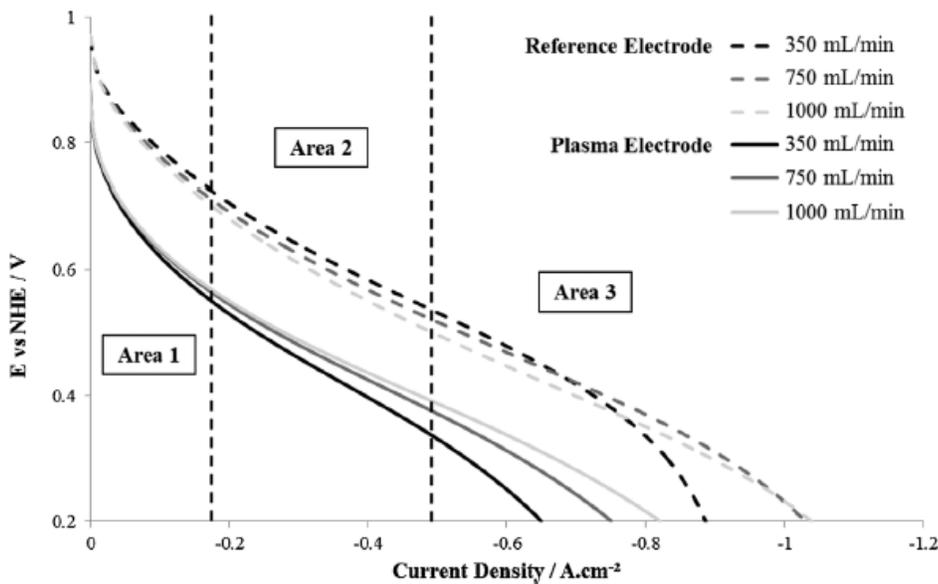
Figure 10. Dynamical polarization curves of the mono-fuel cell containing the reference electrode and the plasma electrode as cathode realized in the following conditions ( $A=25\text{cm}^2$ , open configuration, gap=3 mm,  $Ar=30\text{ L}\cdot\text{min}^{-1}$ , 60W, 300 s).
