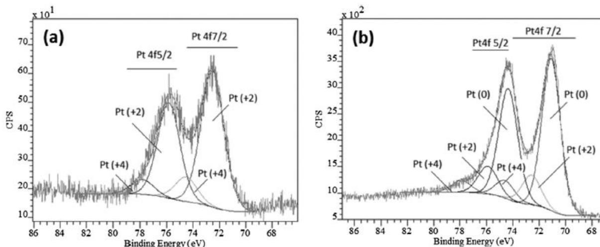
Figure 4. Comparison between Pt 4f spectra for a plasma treatment of the CB/[Pt(acac)<sub>2</sub>] mixture during 300 s (60 W, 30 L.min<sup>-1</sup> Ar, gap=10mm) (a) in the "open configuration" and (b) in the "confined configuration."
