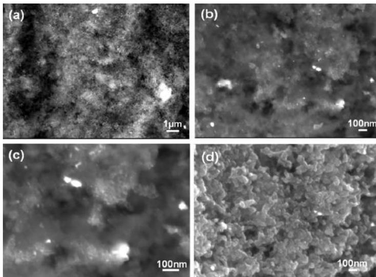
Figure 5. SEM pictures of the CB/ $[\text{Pt}(\text{acac})_2]$  mixture exposed during 300 s to the flowing post-discharge (60 W, gap = 3 mm, Ar flow rate = 30 L/min): (a–c) backscattered electrons, (d) secondary electrons.
