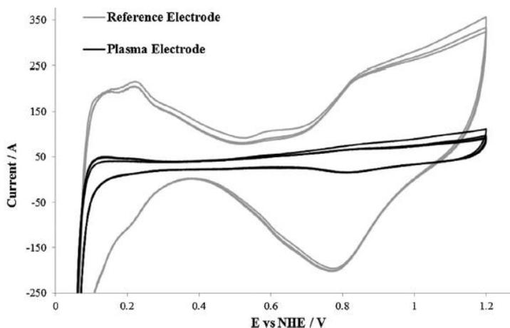
Figure 9. Cyclic voltammogram of the single fuel cell containing the reference electrode (grey) and the plasma electrode (black) as cathode realized in the following conditions ( $A=25 \text{ cm}^2$ , open configuration, gap=3mm,  $\text{Ar}=30 \text{ L}\cdot\text{min}^{-1}$ , 60W, 300 s).
