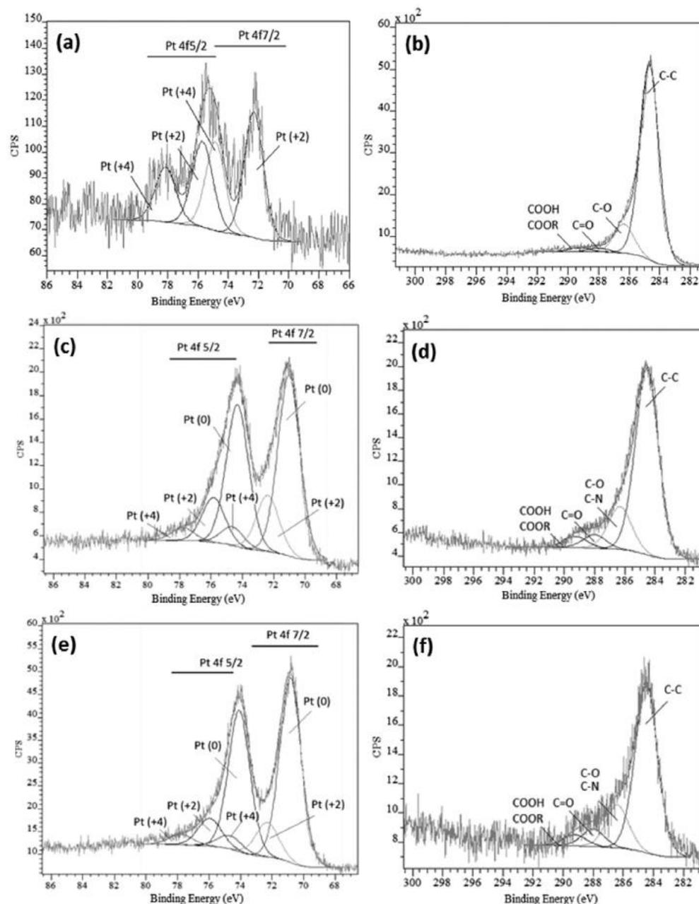
Figure 3. Pt 4f and C 1s XPS peaks for (a, b) CB/[Pt(acac)<sub>2</sub>] untreated mixture (0 s), (c, d) mixture treated for 30 s, and (e, f) mixture treated for 600 s.
