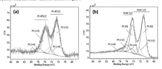
Figure 4. Comparison between Pt 4f spectra for a plasma treatment of the CB/[Pt(acac)<sub>2</sub>] mixture during 300 s (60 W, 30 L.min<sup>-1</sup> Ar, gap=10mm) (a) in the "open configuration" and (b) in the "confined configuration."
