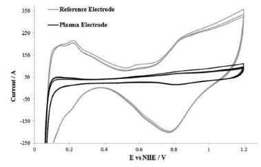
Figure 9. Cyclic voltammogram of the single fuel cell containing the reference electrode (grey) and the plasma electrode (black) as cathode realized in the following conditions (A=25 cm², open configuration, gap=3mm, Ar=30 L.min<sup>-1</sup>, 60W, 300 s).
