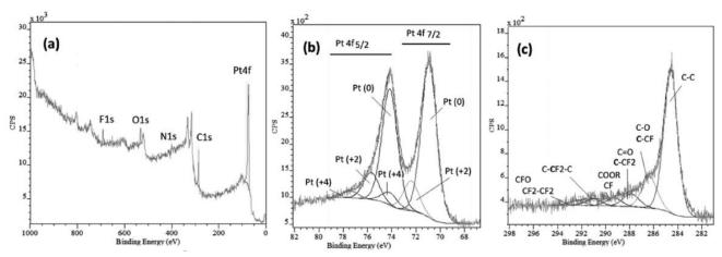
Figure 7. Survey scan of (a) the plasma electrode (open configuration, 300 s, 60 W, 30 L min<sup>-1</sup> Ar), (b) Pt 4f XPS spectra, (c) C 1s XPS spectra.
