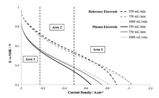
Figure 10. Dynamical polarization curves of the mono-fuel cell containing the reference electrode and the plasma electrode as cathode realized in the following conditions (A=25cm2, open configuration, gap=3 mm, Ar=30 L.min-1, 60W, 300 s).
