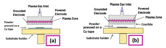
Figure 1. Scheme of the RF plasma torch (Atomflo-250D SurfX) for two configurations:
