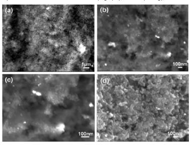
Figure 5. SEM pictures of the CB/[Pt(acac)<sub>2</sub>] mixture exposed during 300 s to the flowing post-discharge (60 W, gap = 3 mm, Ar flow rate = 30 L/min): (a-c) backscattered electrons, (d) secondary electrons.
