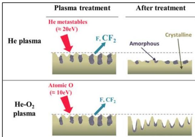
Figure 7. Scheme of the two possible etching processes. In a pure helium plasma, the most important fragment produced is CF<sub>2</sub>.
