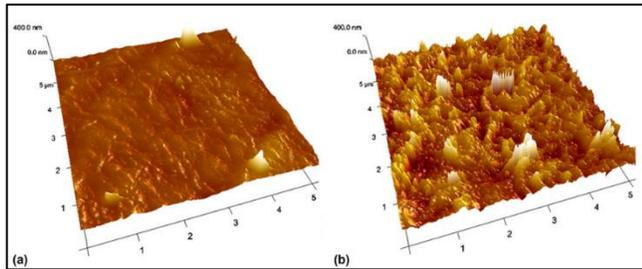
**Figure 4.**  $5 \times 5 \mu\text{m}^2$  AFM 3D images of a PTFE surface treated by (a) pure He plasma ( $R_{\text{RMS}}$  15 nm) and (b) He- $\text{O}_2$  plasma ( $R_{\text{RMS}}$  58 nm), with a Z scale of 511 nm. ( $L_s = 10$  mm,  $v_s = 25$  mm/s,  $g_s = 500$  lm,  $N_s = 1000$ ,  $\Phi(\text{He}) = 15$  L/min,  $\Phi(\text{O}_2) = 0$  and 100 mL/min,  $P = 90$  W).
