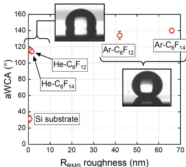
**Figure 10.** Advancing WCA and roughness RMS of the silicon wafer substrate and the pp films. Illustration of the drop behavior of (left) Ar- $\text{C}_6\text{F}_{14}$  and (right) He- $\text{C}_6\text{F}_{12}$  coatings. (0.2 L/min precursor-carrier gas, 5 L/min carrier gas total, 50 W).
