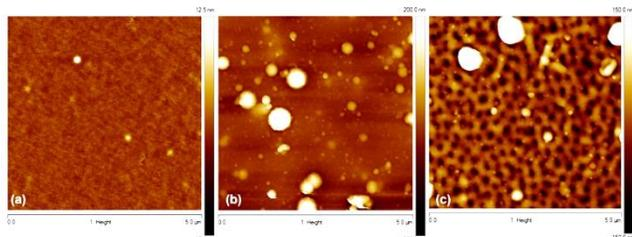
**Figure 11.**  $5 \times 5 \mu\text{m}^2$  AFM images of (a) He- $\text{C}_6\text{F}_{12}$ , (b) Ar- $\text{C}_6\text{F}_{12}$  and (c) Ar- $\text{C}_6\text{F}_{14}$  pp-films. (0.2 L/min  $\text{C}_6\text{F}_{14}$ -carrier gas, 5 L/min carrier gas total, 50 W, thickness of about 300 nm).
