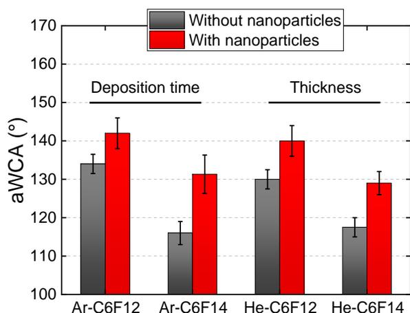
**Figure 12.** Advancing WCA of the pp films without nanoparticles (light gray) and with nanoparticles (red) for an identical deposition time of 2 min (left) and a similar thickness of about 200 nm (right). (0.2 L/min  $C_6F_{12}$ -carrier gas, 5 L/min carrier gas total, 50 W).
