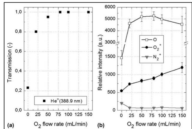
**Figure 6.** (a) Transmission rate of He  $2^3S$  at 388.9 nm and (b) optical emission intensity of O (844.6 nm),  $\text{O}_2^+$  (525 nm) and  $\text{N}_2^+$  (391 nm) in the He- $\text{O}_2$  post-discharge ( $g_s = 1$  mm,  $\Phi(\text{He}) = 15$  L/min,  $P = 120$  W).
