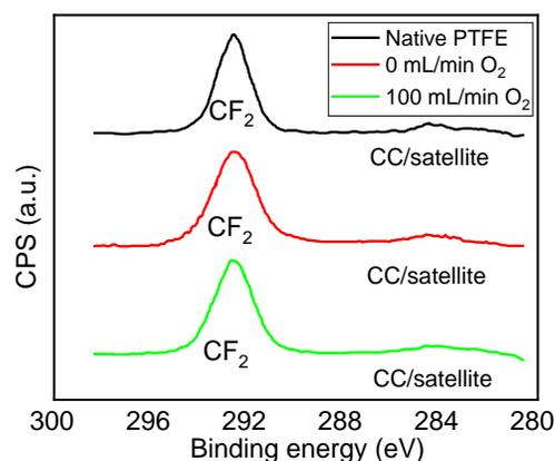
**Figure 3.** HR C 1s spectra of untreated PTFE and He and He-O<sub>2</sub> plasma-treated PTFE. ( $L_s = 10$  mm,  $v_s = 25$  mm/s,  $g_s = 500$   $\mu\text{m}$ ,  $N_s = 1000$ ,  $\Phi(\text{He}) = 15$  L/min,  $\Phi(\text{O}_2) = 0$  and 100 ml/min,  $P = 90$  W).
