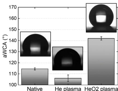
**Figure 2.** Advancing WCAs of untreated PTFE and He and He-O<sub>2</sub> plasma-treated PTFE, with the associated pictures of the static WCA. ( $P = 90$  W,  $L_s = 10$  mm,  $v_s = 25$  mm/s,  $g_s = 500$   $\mu\text{m}$ ,  $N_s = 1000$ ,  $\Phi(\text{He}) = 15$  L/min,  $\Phi(\text{O}_2) = 0$  and 100 ml/min).
