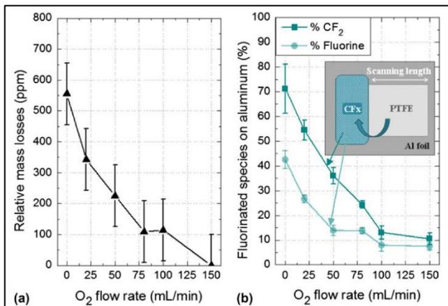
**Figure 5.** (a) Relative mass losses of PTFE as a function of the oxygen flow rate and (b) relative surface composition of the fluorinated fragments ejected from the PTFE on the aluminum foil. ( $L_s = 10$  mm,  $v_s = 25$  mm/s,  $g_s = 1$  mm,  $N_s = 1000$ ,  $\Phi(\text{He}) = 15$  L/min,  $P = 90$  W).
