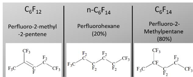
Figure 1. Structures of the two liquid precursors C<sub>6</sub>F<sub>12</sub> and C<sub>6</sub>F<sub>14</sub> and the two C<sub>6</sub>F<sub>14</sub> isomers.
