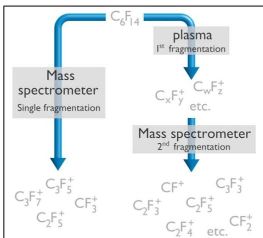
**Figure 9.** Scheme of the possible fragmentation of  $\text{C}_6\text{F}_{14}$  (left) in the mass spectrometer and (right) in the plasma, followed by the mass spectrometer ( $\text{C}_x\text{F}_y^+$  and  $\text{C}_w\text{F}_z^+$  assuming to be  $\text{CF}_3^+$ ,  $\text{C}_3\text{F}_7^+$  and  $\text{C}_3\text{F}_5^+$  according to MS results).
