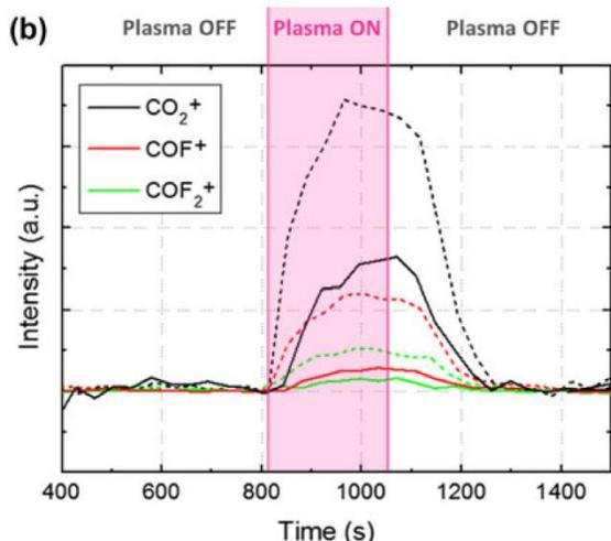
**Figure 8.** Intensity of the (a)  $\text{CF}_3^+$ ,  $\text{C}_2\text{F}_5^+$ ,  $\text{C}_3\text{F}_5^+$  and  $\text{C}_3\text{F}_7^+$  and (b)  $\text{CO}_2^+$ ,  $\text{COF}^+$ ,  $\text{COF}_2^+$  fragments generated during the atmospheric pressure PECVD of  $\text{C}_6\text{F}_{14}$  as a function of time, in argon (full curves) and helium (dashed curves). (0.2 L/min  $\text{C}_6\text{F}_{14}$ -carrier gas, 5 L/min carrier gas total, 50 W).
