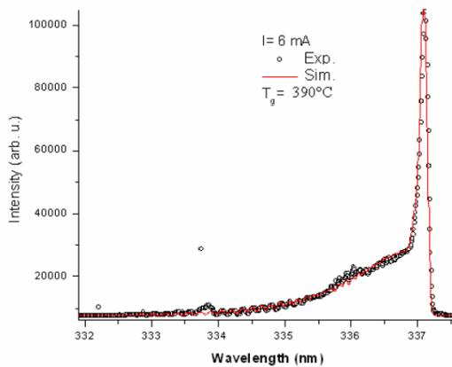
Fig. 6 Fitting of  $N_2$  2<sup>nd</sup> positive system  $C^3II_u-B^3II_g$  (OES) for  $I_d=6$  mA.
