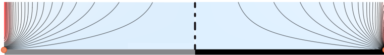
FIGURE 21. Left: Isolines for the radial velocity \tilde{u}_r extracted from the numerical simulations. Right: Theoretical isolines for the radial velocity given by the composite expansion \tilde{u}_r^{\text{comp}} . Note that the transverse scale has here been stretched to visualize the boundary layer.
