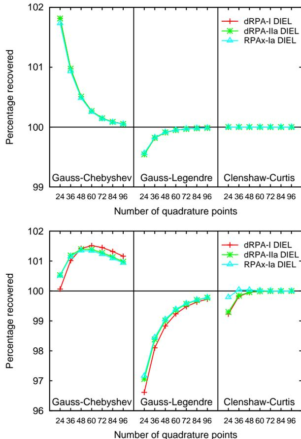
FIG. 1. Convergence with respect to the number of quadrature points of the Gauss-Chebyshev, Gauss-Legendre and Clenshaw-Curtis schemes for Li<sup>+</sup> (up) and Mg (down). The dRPA-I DIEL energy is compared to the dRPA-I PLASMON energy, and the dRPA-IIa DIEL and RPAX-Ia DIEL are compared against their AC analog.
