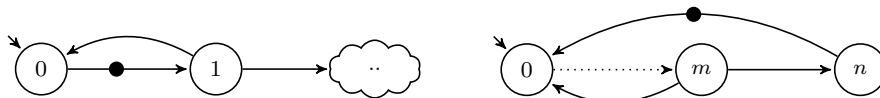
Fig. 5 Worst cases to detect accepting cycle using only one thread. The left automaton is bad for Tarjan since the accepting cycle is always found only after popping state 1. The right one disadvantages Dijkstra since the union of the states represented by dots can be costly.
