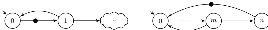
Fig. 5 Worst cases to detect accepting cycle using only one thread. The left automaton is bad for Tarjan since the accepting cycle is always found only after popping state 1. The right one disadvantages Dijkstra since the union of the states represented by dots can be costly.
