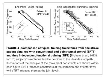
obtained for one subject with both control approaches, along with a representation of associated control approaches.
