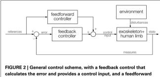
calculates the error and provides a control input, and a feedforward control that directly contains the desired values and provides another control input. Both inputs are combined into a single control fed to the exoskeleton actuators. Measures of the current state are fed back to the controller. The interaction with the environment acts like a disturbance on the exoskeleton control algorithm.
