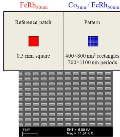
Figure 1. Top: sketch of the sample lithographic preparation, showing the FeRh reference patch and the pattern of  $400 \times 800 \text{ nm}^2$  rectangles etched in the Co/FeRh film. Bottom: scanning electron microscopy image of the pattern (the white scalebar is  $2 \mu\text{m}$ ).
