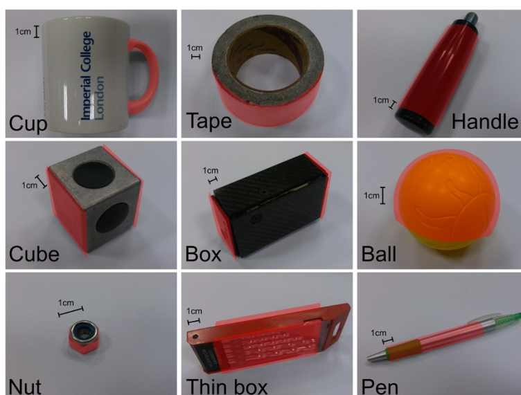
Figure 4 The nine objects used for the experiments: the handle of a mug, a large tape toll, a handle, a 4 cm metallic cube, a 300 grams parallelepiped box, a hollow plastic ball, a M12 nut, a thin rectangular drill bits box and finally a ballpen. The experimenter instructed the subject to grasp the areas of interest highlighted in red.
