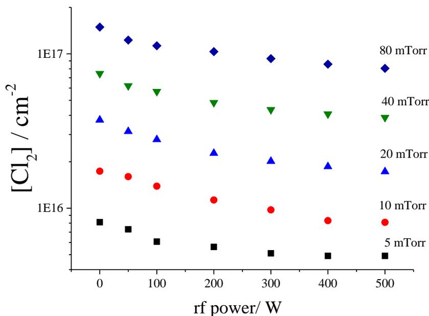
Figure 8 Line-integrated Cl<sub>2</sub> density in the discharge ( $p = 5 - 80$  mTorr,  $P = 0 - 500$  W).
