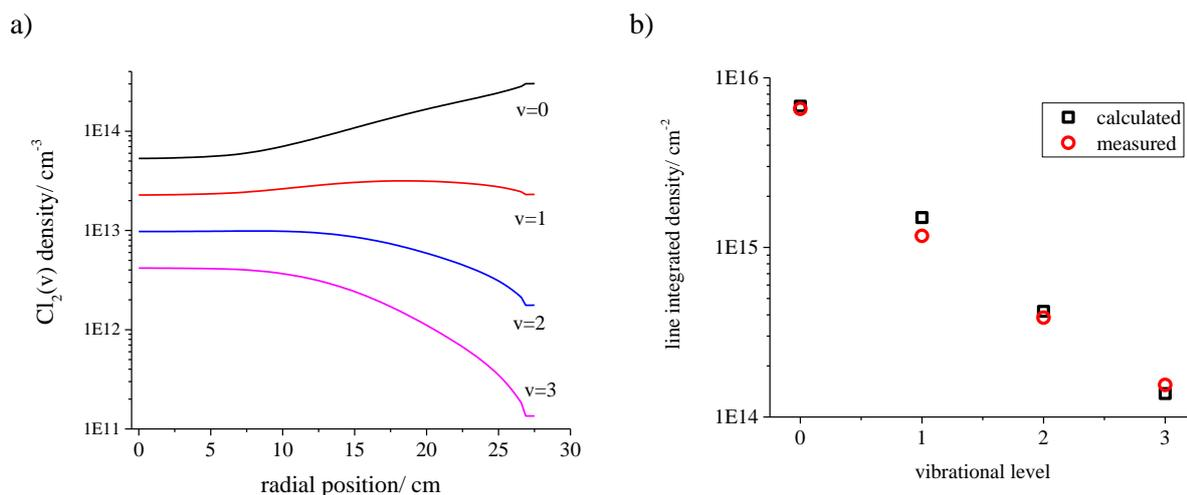
Figure 11 a) Radial profiles of densities of  $\text{Cl}_2(v=0-3)$  calculated assuming local thermodynamic equilibrium of heavy plasma species. b) Comparison between measured and calculated line-integrated densities of  $\text{Cl}_2(v=0-3)$ .
