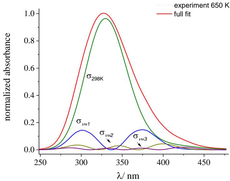
Figure 4 Normalized experimental absorption spectrum of  $\text{Cl}_2$  at  $T_{\text{cell}} = 650 \text{ K}$  (dotted line) and the corresponding fit. Contributions of individual vibrational states are depicted separately.
