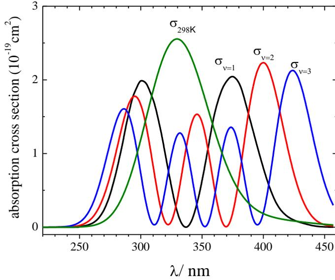
Figure 2 Partial absorption cross sections used for fitting of experimental data.
