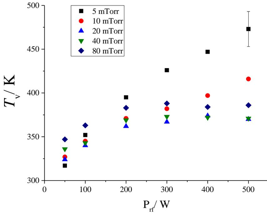
Figure 9 Effective vibrational temperature (from the ratio of populations in  $v=1/v=0$ ) of  $Cl_2$  as a function of the rf power measured at various gas pressures. An uncertainty of ( $\pm 20$  K) is estimated in the  $T_v$  determination from the standard deviation of 7 independent measurements.
