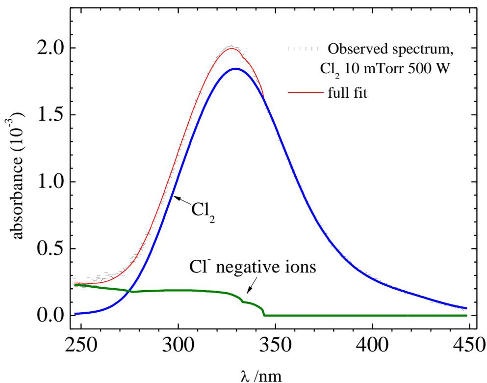
Figure 7 Absorption spectrum of  $\text{Cl}_2$  plasma ( $p = 10$  mTorr,  $P = 500$  W) and the corresponding fit. Contributions of  $\text{Cl}_2$  molecules and  $\text{Cl}^-$  ions are shown separately. The best-fit value of the line-integrated density of negative ions is  $[\text{Cl}^-] = 1.3 \cdot 10^{13} \text{ cm}^{-2}$ .
