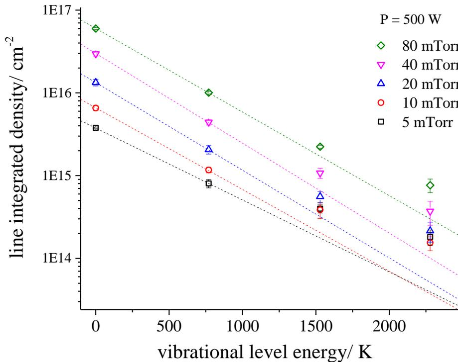
Figure 10 Line integrated densities of  $Cl_2$  ( $v=0-3$ ) measured at different pressures and a fixed rf power  $P = 500$  W. Dashed lines represent Boltzmann distributions with the temperature equal to  $T_v$ . Error bars correspond to the standard deviation of 7 independent measurements.
