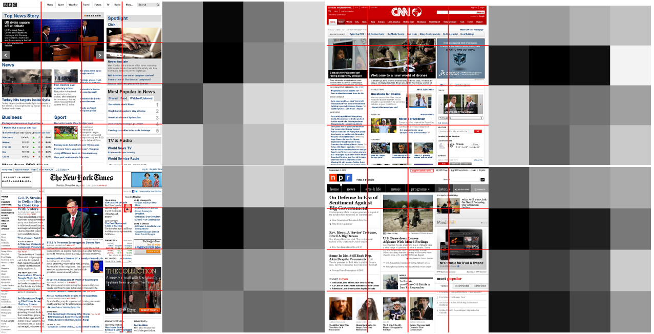
Fig. 6 Important change maps for the homepages of BBC, CNN, New York Times and NPR. (left) Webpage screenshot with webpage regular segmentation blocks (red lines). (right) Absolute values of the eigenvector of the dominant eigenvalue of the distance non-diagonal matrix learned by our method with versions crawled during 5 days and without human supervision (higher values are darker).
