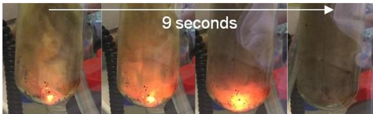
Figure S11. Four snapshots of the reaction forming VC nanoparticles on ac-C.
