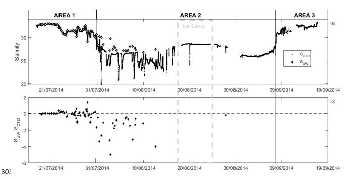
**Figure 3:** Comparison of underway salinity ( $S_{UW}$ ) data with salinity data from surface CTD casts ( $S_{CTD}$ ). a)  $S_{UW}$  is shown in black dots and  $S_{CTD}$  in white diamonds. b) Salinity residuals ( $S_{UW}$ - $S_{CTD}$ ). Data corresponding to Area1 (ice-free outbound), Area2 (Arctic, ice-covered), and Area3 (ice-free return leg) are delimited by the vertical solid lines and the ice camp by the vertical dotted lines.
