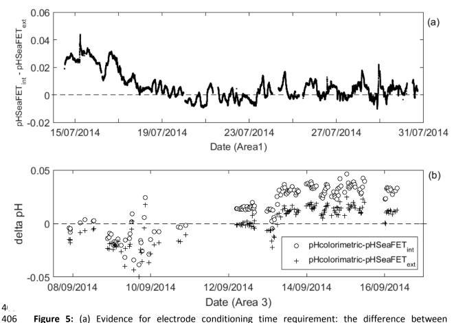
**Figure 5:** (a) Evidence for electrode conditioning time requirement: the difference between pH\_SeaFET\_int and pH\_SeaFET\_ext overtime in Area1; (b) Evidence for internal reference drift: the difference between pH\_colorimetric and pH\_SeaFET\_int/ext overtime in Area3.
