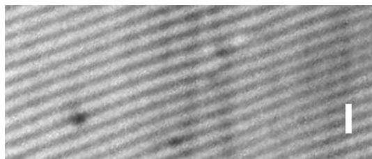
Fig. 5 Photomicrograph of oily streaks having concentration c = 5 wt% of the left-handed chiral dopant ZLI-811. Notice that the rotation of the oily streaks has a sense opposite that of the right-handed dopant CB15 in Fig. 4. Bar corresponds to 2 \mu\text{m} and is parallel to the easy axis.
