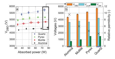
Figure 6. (a) RMS applied voltage ( $V_{DBD}$ ) as a function of absorbed power for four different dielectric materials at f = 27 kHz, and (b) RMS voltage components as a function of the dielectric material at a given absorbed power  $P_{abs} = 75$  W;  $\Phi(CO_2) = 200$  mL<sub>n</sub> · min<sup>-1</sup>. The relative permittivities of the materials are indicated with crosses, referring to the right y-axis.
