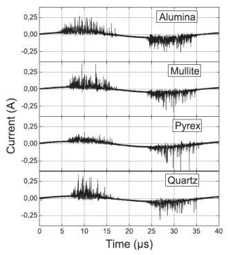
Figure 7. Current profiles as a function of time for four different dielectric materials;  $P_{abs} = 75 \text{ W}$ ;  $\Phi(CO_2) = 200 \text{ mL}_n \cdot \text{min}^{-1}$ .
