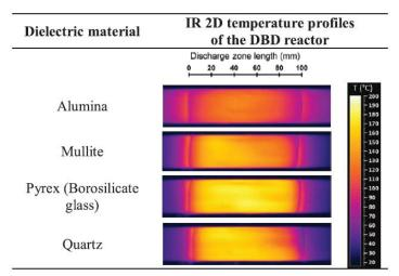
Figure 9. 2D temperature profiles of the DBD reactors for the four different dielectric materials, for P<sub>abs</sub> = 75 W, process time = 4 min. The black graded line indicates the length of the outer electrode, i.e. the discharge region.
