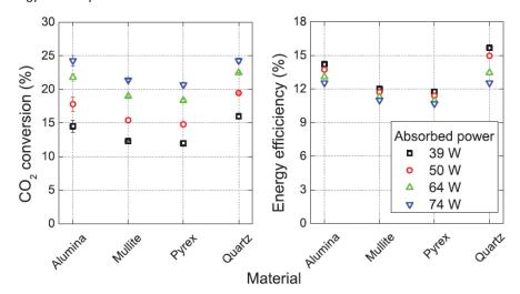
Figure 5. (a) CO<sub>2</sub> conversion and (b) energy efficiency for different values of the absorbed power and for four different dielectric materials; f = 27.1kHz;  $\Phi(CO_2) = 200 \text{ mL}_n \cdot \text{min}^{-1}$ .
