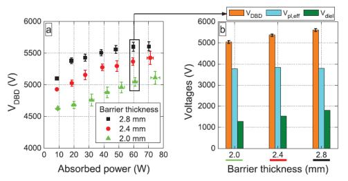
Figure 3. (a) Applied voltage (VDBD) as a function of absorbed power for three different dielectric thicknesses, and (b) voltage components as a function of the dielectric thickness at a given absorbed power  $P_{abs} = 60$  W; f = 28.6 kHz;  $\Phi(CO_2) = 200$  mL<sub>n</sub> · min<sup>-1</sup>.
