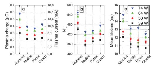
Figure 8. (a) Plasma charge accumulation during one period, (b) number of microdischarges during one period and (c) mean lifetime of the microdischarges, for the four different dielectric materials and for different absorbed powers and  $\Phi(CO_2) = 200 \text{ mL}_n \cdot \min^{-1}$ .
