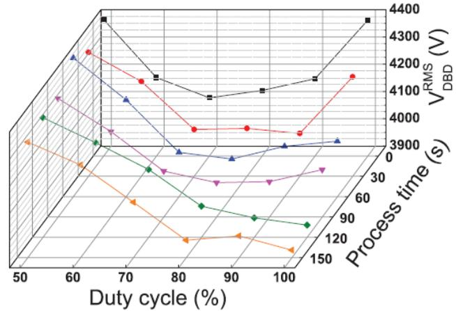
Figure 6. RMS value of the DBD voltage as a function of the duty cycle and the process time.  $P_{\text{applied}} = 50 \text{ W}$ ,  $f_{\text{signal}} = 28.6 \text{ kHz}$ ,  $f_{\text{repetition}} = 500\text{--}900 \text{ Hz}$  and  $\Phi(\text{CO}_2) = 200 \text{ mL}_n \cdot \text{min}^{-1}$ .
