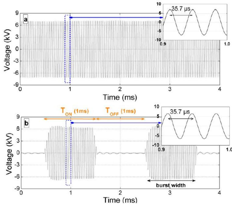
Figure 2. High voltage signals applied to the discharge, with frequency of 28.6 kHz (or period of 35.7 μs), in (a) pure AC mode, and (b) burst mode, with a duty cycle of 50% ( $T_{ON} = T_{OFF} = 1$  ms).
