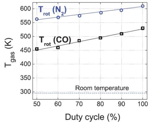
Figure 7. Gas temperature as a function of duty cycle, as obtained from the FPS of N<sub>2</sub> and from the Angstrom CO band; P<sub>applied</sub> = 50 W, f<sub>signal</sub> = 28.6 kHz, f<sub>repetition</sub> = 500–900 Hz and Φ(CO<sub>2</sub>) = 200 mL<sub>n</sub> · min<sup>-1</sup>.
