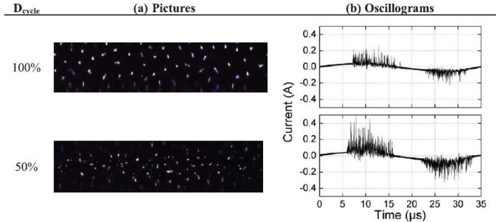
Figure 8. (a) Pictures of the distribution of the microdischarges in the DBD, and (b) corresponding current oscillograms, for two different duty cycles (50 and 100%).  $P_{\text{applied}} = 50 \text{ W}$ ,  $f_{\text{signal}} = 28.6 \text{ kHz}$  and  $\Phi(\text{CO}_2) = 200 \text{ mL}_n \cdot \text{min}^{-1}$ . Camera aperture is 1/100 s.
