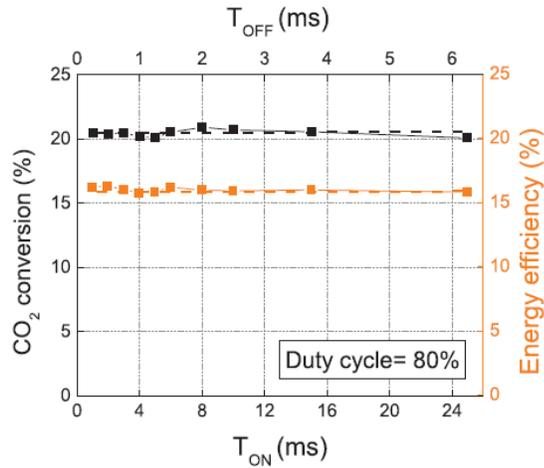
Figure 5.  $\text{CO}_2$  conversion and energy efficiency for a fixed duty cycle of 80%, as a function of  $T_{\text{ON}}$ .  $P_{\text{applied}} = 50 \text{ W}$ ,  $f_{\text{signal}} = 28.6 \text{ kHz}$  and  $\Phi(\text{CO}_2) = 200 \text{ mL}_n \cdot \text{min}^{-1}$ .
