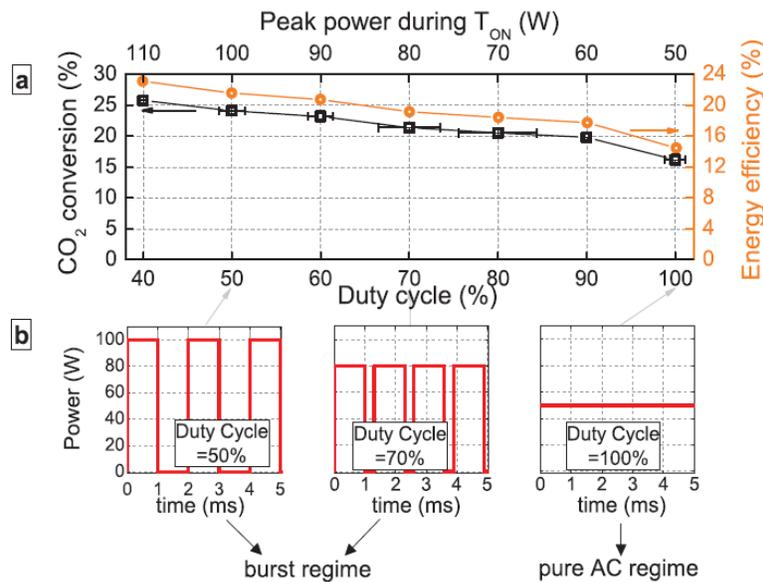
Figure 4. (a) CO<sub>2</sub> conversion and energy efficiency as a function of the duty cycle —  $P_{\text{applied}} = 50 \text{ W}$ ,  $f_{\text{signal}} = 28.6 \text{ kHz}$ ,  $f_{\text{repetition}} = 400\text{--}900 \text{ Hz}$  and  $\Phi(\text{CO}_2) = 200 \text{ mL}_n \cdot \text{min}^{-1}$ ; (b) power versus time for  $D_{\text{cycle}} = 50, 70$  and  $100\%$ .
