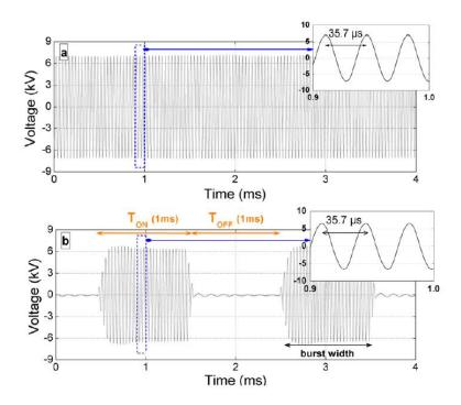
Figure 2. High voltage signals applied to the discharge, with frequency of 28.6 kHz (or period of 35.7  $\mu$ s), in (a) pure AC mode, and (b) burst mode, with a duty cycle of 50% ( $T_{ON} = T_{OFF} = 1$  ms).
