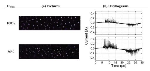
Figure 8. (a) Pictures of the distribution of the microdischarges in the DBD, and (b) corresponding current oscillograms, for two different duty cycles (50 and 100%).  $P_{applied} = 50 \text{ W}$ ,  $f_{signal} = 28.6 \text{ kHz}$  and  $\Phi(CO_2) = 200 \text{ mL}_n \cdot \text{min}^{-1}$ . Camera aperture is 1/100 s.
