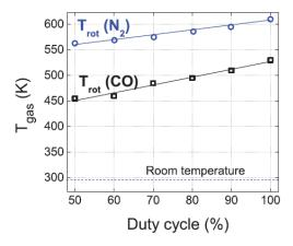
Figure 7. Gas temperature as a function of duty cycle, as obtained from the FPS of  $N_2$  and from the Angstrom CO band;  $P_{applied} = 50 \text{ W}$ ,  $f_{signal} = 28.6 \text{ kHz}$ ,  $f_{repetition} = 500-900 \text{ Hz}$  and  $\Phi(CO_2) = 200 \text{ mLn} \cdot \text{min}^{-1}$ .
