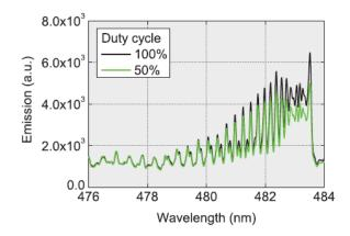
Figure 3. CO band from the  $[B_1\Sigma^+ \to A^1\Pi; v' = 0 \to v'' = 1]$  Angstrom System in the DBD supplied with pure CO<sub>2</sub>, at two different duty cycles.
