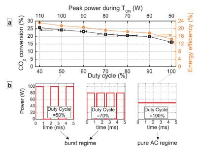
Figure 4. (a) CO<sub>2</sub> conversion and energy efficiency as a function of the duty cycle —  $P_{applied}$  = 50 W,  $f_{signal}$  = 28.6 kHz,  $f_{repetition}$  = 400–900 Hz and  $\Phi(CO_2)$  = 200 mL<sub>n</sub> · min<sup>-1</sup>; (b) power versus time for  $D_{cycle}$  = 50, 70 and 100%.
