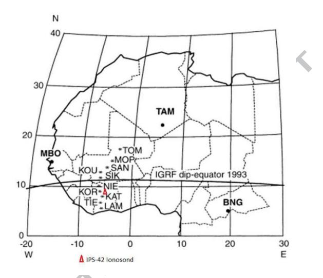
Figure 2: The 5°W meridian chain magnetic stations (asterisk) and the ionosonde (triangle) installed in West Africa during the International Equatorial Electrojet Year (IEEY).
