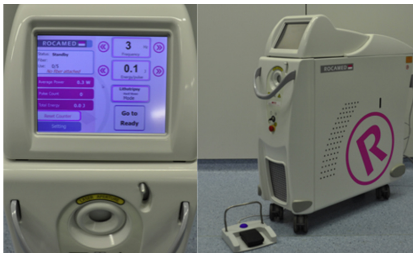
Fig. 9. A Holmium-YAG 30W laser lithotripter (Rocamed).
