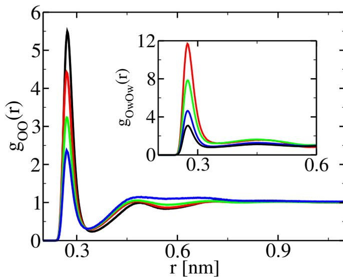
Fig.3 - Site-site correlations in ethanol-alkane mixtures. Main panel: ethanol oxygen-oxygen correlation function. Inset: methyl-methyl correlation (blue for pentane, green for benzene and red for hexane). Color convention according to ethanol mole fraction as in Fig.2.
