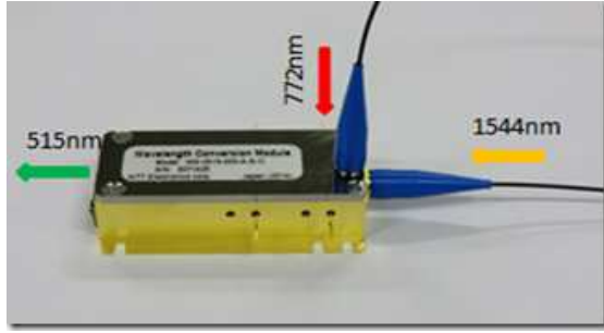
Fig. 2. Photograph of the SFG – PPLN waveguide module
