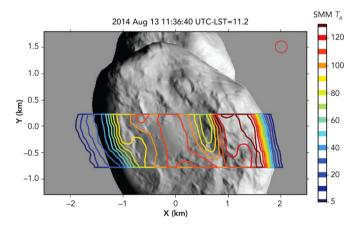
**Fig. 11.** A partial map of the temperature of the nucleus of comet 67P/Churyumov–Gerasimenko, from the submillimetric continuum observations of MIRO on *Rosetta*, superimposed on the model of its shape deduced from imaging in the visible [25]. It can be seen on the left side that MIRO observes the night side, for which visible imaging provides no information. The temperatures vary, following solar insolation, from about 30 K (night side) to 130 K. The comet was then at 3,5 AU from the Sun.
