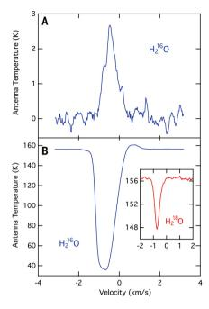
**Fig. 10.** An example of the water lines observed at 0.5 mm wavelength in comet 67P/Churyumov–Gerasimenko with MIRO on *Rosetta* [25]. Top: observation on 23 June 2014 at a distance of 128 000 km. Bottom: observation on 19 August 2014 at a distance of 81 km; the lines are then seen in absorption against the continuum of the nucleus.
