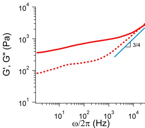
Fig. 6: Elastic (full line) and loss (dotted line) moduli of a home made collagen gel of concentration  $4\text{mg.mL}^{-1}$ . The data was obtained from two beam fitting of fluctuation spectra. The corresponding value of surface tension is  $52\text{mN.m}^{-1}$ . The solid blue line represents a power law with an exponent  $3/4$ .
