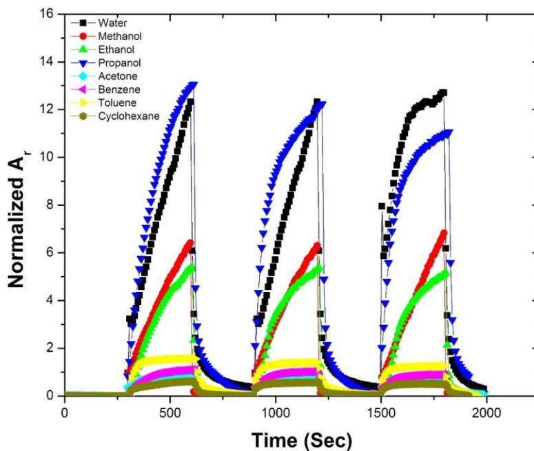
Figure 4. Effect of flow rate of different vapours on the amplitude  $A_r$  of linear polyamide based on  $\beta$ -CD(OH)<sub>19</sub>(NH<sub>2</sub>)<sub>2</sub>-CNT sensor.
