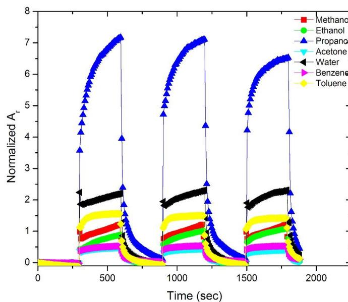
Figure 6. Effect of flow rate of different vapours on the amplitude  $A_r$  of branched polyamide based on  $\beta$ -CD(OH)<sub>14</sub>(NH<sub>2</sub>)<sub>7</sub>-CNT sensor.
