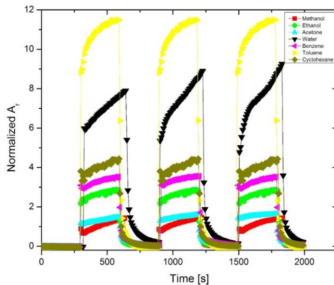
Figure 5. Effect of flow rate of different vapours on the amplitude  $A_r$  of linear polyamide based on  $\beta$ -CD(OBn)<sub>19</sub>(NH<sub>2</sub>)<sub>2</sub>-CNT sensor.
