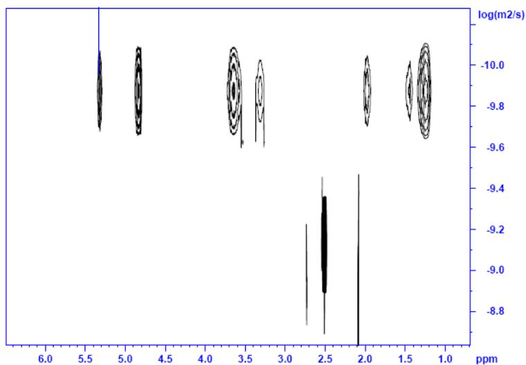
Figure 3: DOSY NMR spectrum of the polycondensate synthesized from the (Z) octadec-9-enedioic-N-hydroxysuccinimide ester and  $\beta$ -CD(NH<sub>2</sub>)<sub>2</sub>(OH)<sub>19</sub> in DMSO at 25°C.
