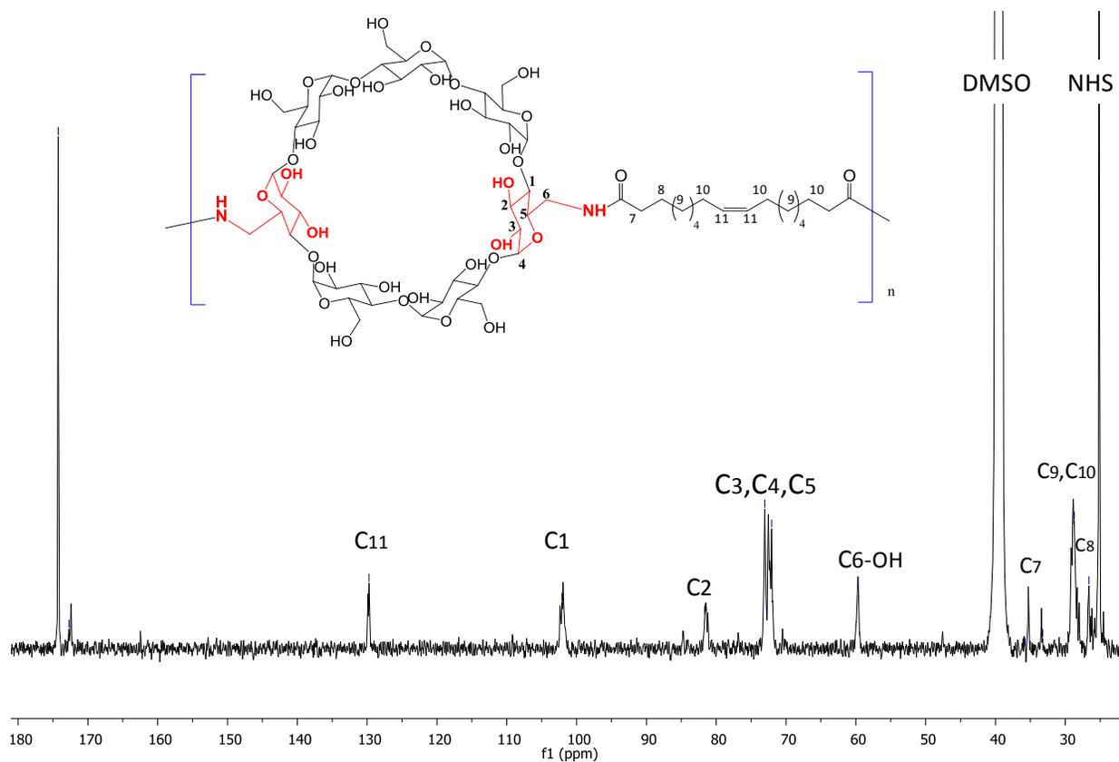
Figure 2:  $^{13}\text{C}$  NMR of the polycondensate synthesized from the (Z) octadec-9-enedioic-N-hydroxysuccinimide ester and  $\beta\text{-CD}(\text{NH}_2)_2(\text{OH})_{19}$  in DMSO at  $25^\circ\text{C}$ .
