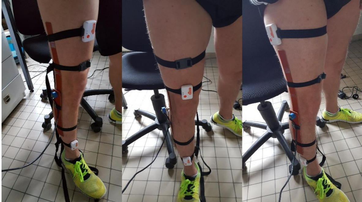
Figure 4. Tested sensor positions ( Left: Sensor on the thigh directly; Middle: Sensor above the kneecap; Right: Sensor in the sagittal plane).
