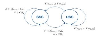
Fig. 5: The two modes of the hybrid spectrum sharing
