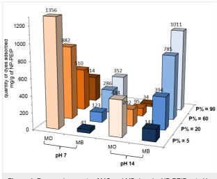
**Figure 4:** Removed amounts of MO and MB dyes by NP-PEIP*x* at pH 7 and 14. P% significantly affects adsorption of MB and MO. At neutral pH, much more MO is eliminated than MB, while the contrary is observed at basic pH.
