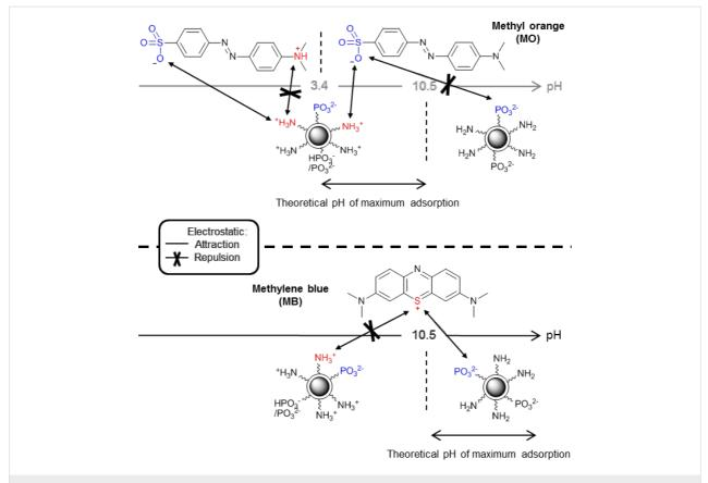
**Figure 3:** Prediction of the best range of pH values for electrostatic attractions between NP-PEIP and MO and MB dyes. Only the major interaction (i.e., ammonium) is represented. For MO, an interaction occurs with sulphates and ammonium groups, until the  $pK_a$  (NH<sub>3</sub><sup>+</sup>/NH<sub>2</sub>) is reached. Cationic MB is attracted by the phosphonate groups introduced on PEI at basic pH values.
