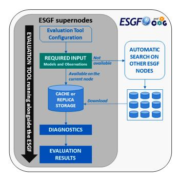
**Figure 5.** Schematic diagram of the envisaged evaluation tool processing stream for CMIP6. The schematic displays how the tools will be executed directly on ESGF supernodes exploiting optimized ESGF data organization and software solutions (see details in Sect. 2.3).
