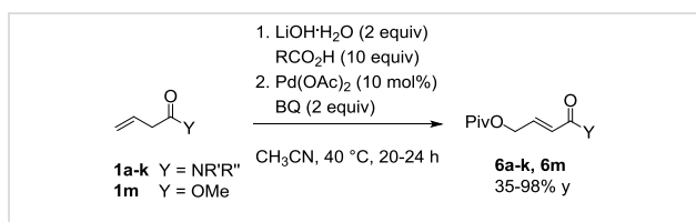
Scheme 4 Pd(II)-catalyzed allylic pivaloxylation. c Reaction conditions: pivalic acid (10.0 equiv), LiOH·H 2 O (2.0 equiv), Pd(OAc) 2 (10 mol%), BQ (2.0 equiv), 1 (1.0 equiv), CH 3 CN (0.2 M).
