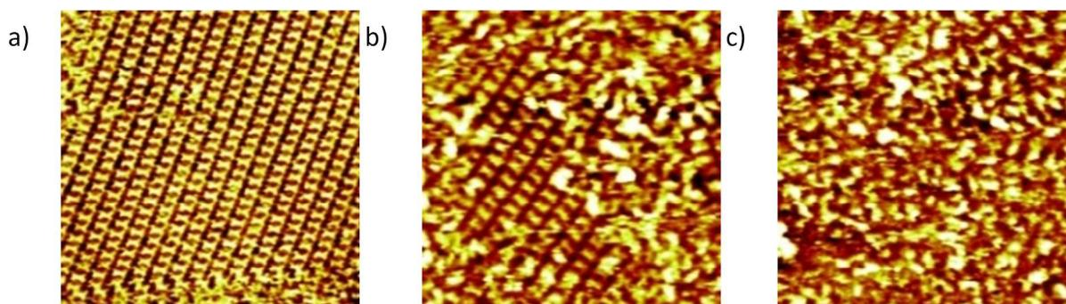
Figure 1. STM images at the liquid/HOPG interface at room temperature, a) 1:4 mixture of Janus tecton and pedestal molecule (60 nm x 60 nm,  $I_t = 8.6$  pA,  $V_t = -1320$  mV), b) 1:1 mixture of Janus tecton and pedestal molecule (50 nm x 50 nm,  $I_t = 9.9$  pA,  $V_t = -1602$  mV), c) Janus tecton solution (50 nm x 50 nm,  $I_t = 8.6$  pA,  $V_t = -1596$  mV).
