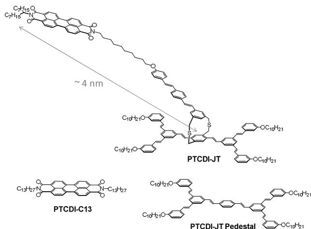
Scheme 1: Schematic structures of the two-faced Janus tecton PTCDI-JT, PTCDI-JT pedestal and *N,N'*-ditridecyl-3,4,9,10-perylenedicarboximide PTCDI-C13 molecules. The distance between the end of the fluorescent unit and the dithiaparacyclophane bridge in PTCDI-JT is typically  $\sim 4$  nm
