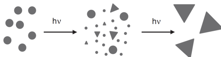
Figure 38: At the early stages of the synthesis, nanoplates and spherical particules are formed. The clusters dissolve and redeposit on the nanotriangles that act as seeds for further growth. From ref.336. Reprinted with permission from AAAS.
