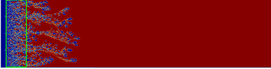
Fig. 15 Injection of an intermediate-viscosity fluid as a second step in a rectangular domain (injection from the left-hand side), case B. (with diffusion). In blue the phase containing both fluids 1 and 2, in red fluid 0. Inside the rectangle, fluid 0 is mobilized by fluid 2, compared to Figure 14 and thus the receding-fluid ratio decreases inside this slice of porous medium compared to the single-step case
