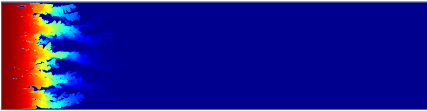
Fig. 16 Same simulation as in the previous Figure. In this figure, the receding fluid is in blue, and the mixture of advancing fluids is plotted with a color palette representing the mixture concentration c , varying from for c = 1 (pure fluid 2) to blue for (pure fluid 1 or pure fluid 0)
