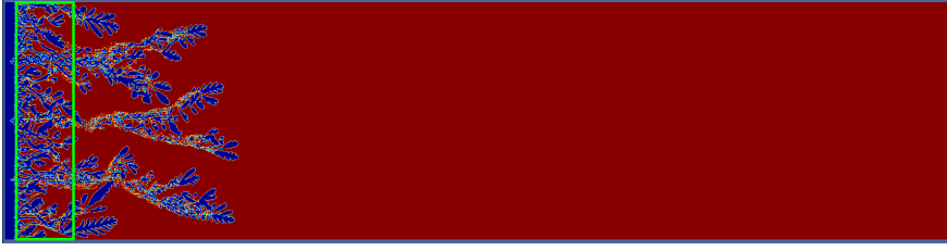
Fig. 14 Invasion of a porous medium by a single low-viscosity fluid. As no intermediate-viscosity fluid is injected, the high-viscosity fluid is not mobilized much inside the rectangle.
