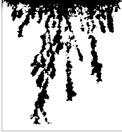
Fig. 1 2D imaging of waterflood in Bentheimer sandstone with 2.0 \text{ kg.m}^{-1} \cdot \text{s}^{-1} crude oil. Water is injected from the top, in black is the injected water. From Skauge et al. (2012) after applying a threshold to the image
